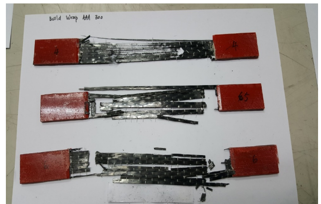
Sample Tested: CFRP Wrap for 300gm/m 2
