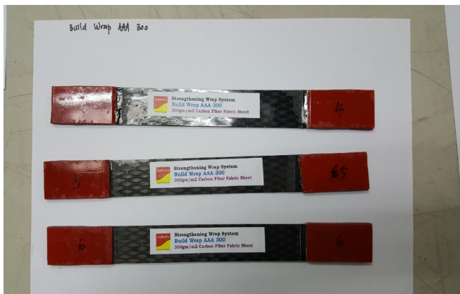
Specimen Sample: CFRP Wrap for 300gm/m 2
